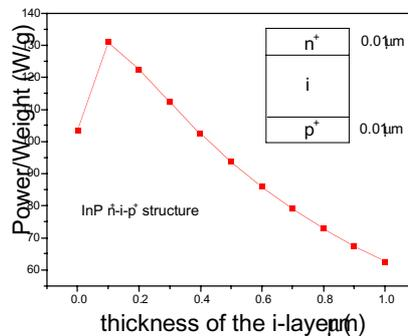
Fig.6 The relationship between power/weight of  $n^+i-p^+$  InP solar cell and the thickness of the i-layer
