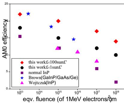
Fig.3 Comparison of radiation hardness of several structures
