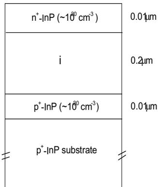
Fig.1 Sketch of the  $n^+i-p^+$  InP solar cell
