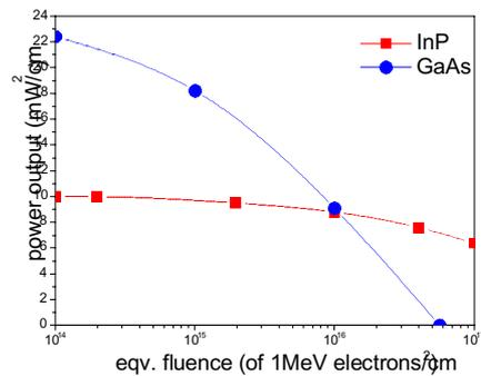
Fig.4 The influence of radiation to power output of GaAs and normal InP solar cells
