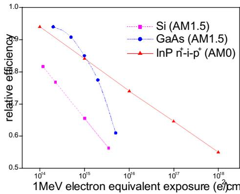
Fig.2 The comparison of relative efficiency of Si, GaAs and  $n^+i-p^+$  InP solar cells
