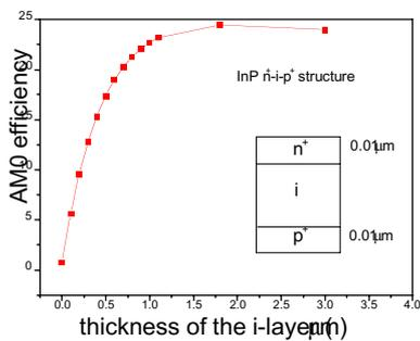
Fig.5 The relationship between AM0 efficiency of  $n^+i-p^+$  InP solar cell and the thickness of the i-layer
