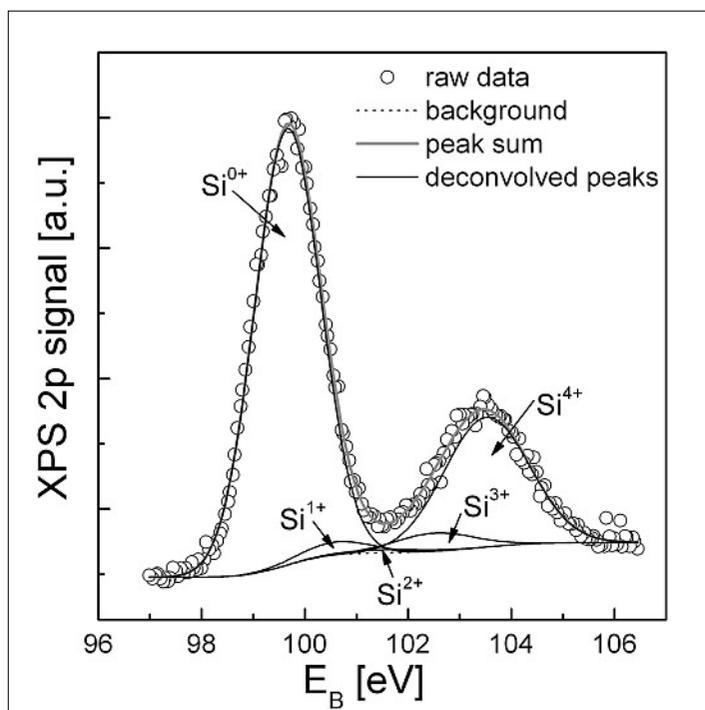
Fig. 2. Line shape analysis with a Shirley background elucidating contributions mainly from the oxidation states  $\text{Si}^{0+}$  and  $\text{Si}^{4+}$ , corresponding to Si and  $\text{SiO}_2$ , respectively. Minor amounts of  $\text{Si}^{1+}$ ,  $\text{Si}^{2+}$  and  $\text{Si}^{3+}$  are revealed. Relative peak areas:  $\text{Si}^{0+}$ : 67.8%,  $\text{Si}^{1+}$ : 2.1%,  $\text{Si}^{2+}$ : 0.6%,  $\text{Si}^{3+}$ : 3.3%,  $\text{Si}^{4+}$ : 26.2%.
