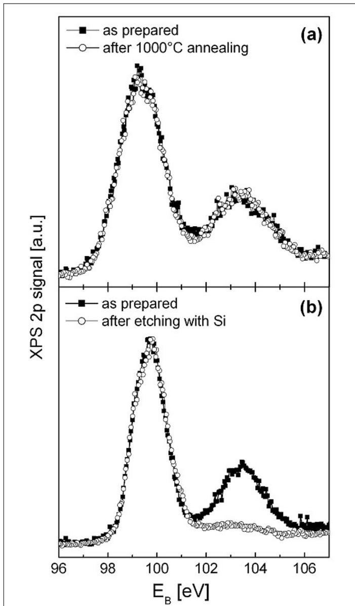
Fig. 4. Si 2p XPS spectra of the oxidized Si(111) wafer (a) before and after UHV annealing for 10 min at  $T_{\text{sub}} = 1000$  °C, (b) before and after thermal deposition of 1 nm Si at  $T_{\text{sub}} = 850$  °C at  $0.1 \text{ \AA/s}$ .
