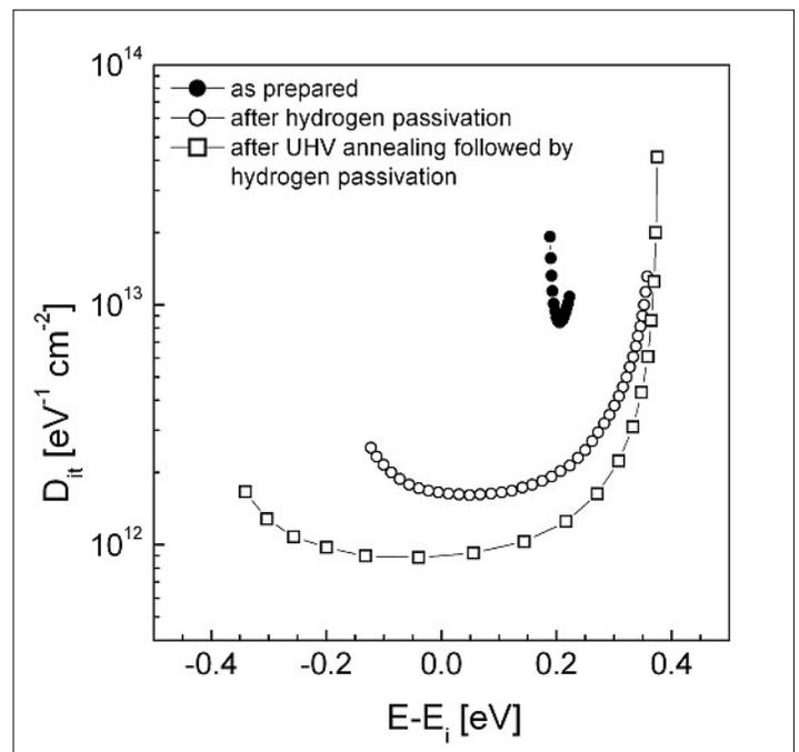
Fig. 5. Distribution of the density of states at the  $\text{SiO}_2/\text{Si}(111)$  interface  $D_{\text{it}}$  relative to the Fermi level  $E_i$  of intrinsic Si as determined from field-dependent SPV measurements ( $t_{\text{ox}} \approx 2$  nm).
