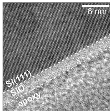
Fig. 3. High-resolution TEM image of the cross-section of the ultrathin  $\text{SiO}_2$  layer on Si(111) with a uniform thickness of 2 nm
