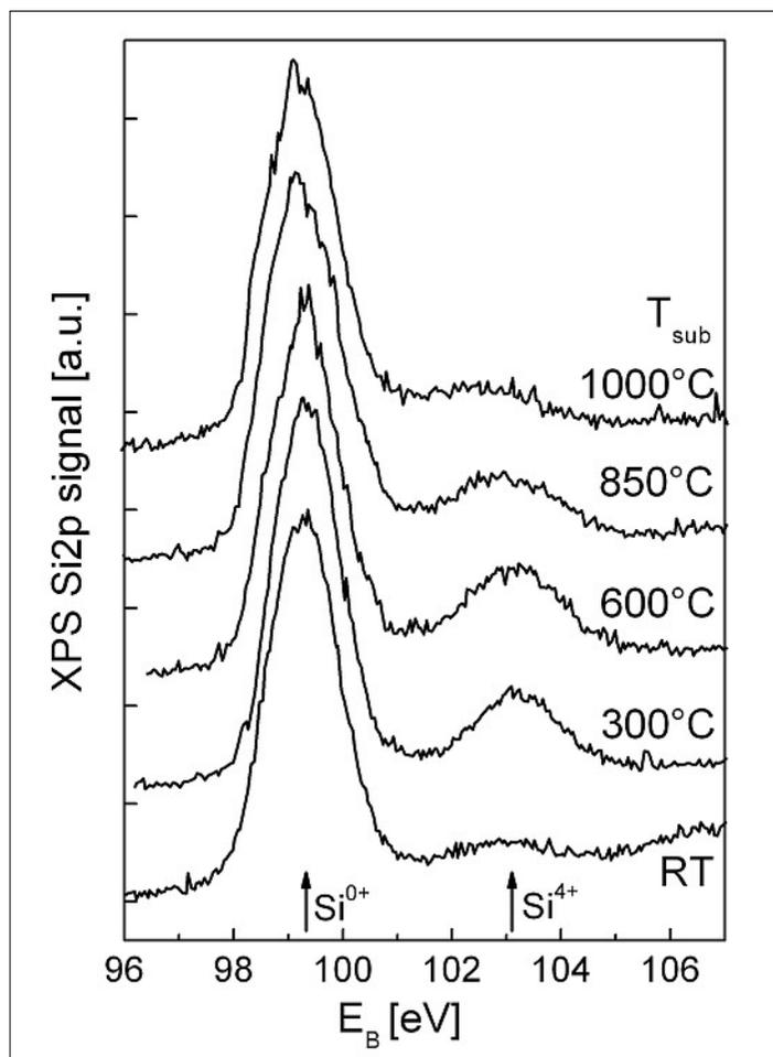
Fig. 1. Si 2p XPS spectra of the Si(111) wafer after RF plasma oxidation with thermalized neutral oxygen atoms at different substrate temperatures ranging from room temperature (RT) to 1000 °C. Oxidation parameters:  $P_{\text{RF}} = 300\text{--}400$  W,  $t = 15$  min.
