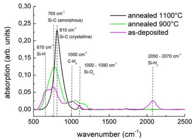
**Figure 1:** FTIR spectra of as-deposited and at various temperatures rapid thermal annealed SRSiC thin films.
