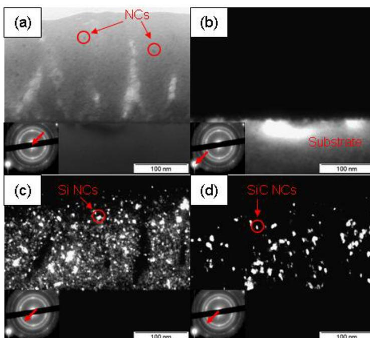
**Figure 4:** (a) Bright field image of SRSiC layer annealed at 1100°C. (b) Dark field image of SRSiC layer, acquired with the Si (200) reflection of the Si Substrate. (c) Dark-field image showing (111) oriented Si nanocrystals. The image was acquired with the Si (111) reflection. (d) Dark-field image acquired with SiC (111) reflection of (111) oriented SiC nanocrystals within the annealed SRSiC layer.
