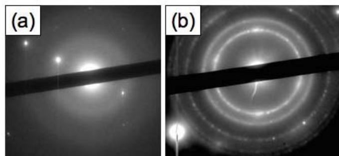
**Figure 3:** Energy filtered Ring Diffraction Patterns of (a) as-deposited SRSiC single layer and (b) annealed SRSiC single layer.
