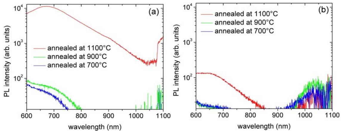
**Figure 5:** (a) Photoluminescence spectra of SRSiC single layers directly after annealing. (b) PL spectra of SRSiC single layers after annealing and H passivation.
