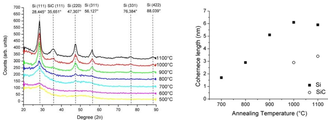
**Figure 2:** (left side) GIXRD measurement of SRSiC single layers annealed at different temperatures. (right side) Mean coherence length of Si and SiC NCs as a function of annealing temperature.
