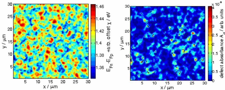
**Figs. 4,5:** Lateral scans of fluctuation in quasi-Fermi level splitting (left) and of defect absorption  $A_{\text{Def}}$  resulting from sub gap absorption (right).
