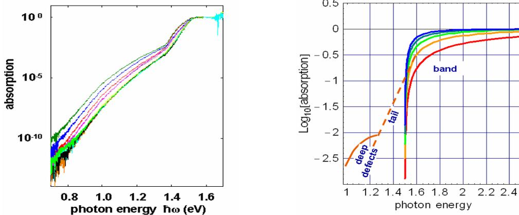
**Figs. 2, 3:** Experimentally detected local absorptions exemplarily plotted for 5 different positions (lateral resolution  $\leq 1 \mu\text{m}$ ) (left) and artificial assembly of absorption of an ideal direct semiconductor degraded additionally by contributions from tail and deep gap states (right).
