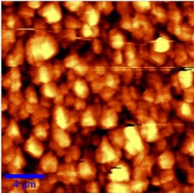
**Figs. 1a:** AFM-scan for demonstrating thickness fluctuations (surface roughness) of a typical polycrystalline  $\text{Cu}(\text{In,Ga})\text{S}_2$  absorber ( $d_{\text{CIGS}_2} = 2 \mu\text{m}$ ).
