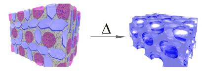
**Scheme 1.** Scheme of formation of crystalline mesoporous titania films (right side) via the "brick and mortar" approach. The nanocrystalline titania "bricks" (light blue, left side) are dispersed in amorphous titania "mortar" (grey), which is periodically self-assembled around the micelles of the polymer template (magenta).
