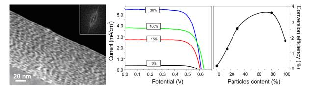
**Figure 2.** Left: Cross-sectional STEM-HAADF image of a film made from 50 % nanoparticles and Fourier transform of the picture revealing the periodic pore structure (inset). Middle: Photocurrent-voltage curve of "brick and mortar" titania layers with varying nanoparticle content. Right: Dependence of conversion efficiency of DSC devices on the nanoparticle content of the "brick and mortar" titania layers (Layer thickness 1.0 µm, D205 sensitizer and Z646 non-volatile electrolyte).
