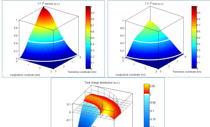
Scheme: Charge distribution between a core and a shell
