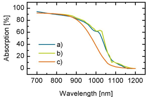
Figure 2: Simulated absorption curves of a 40  $\mu\text{m}$  thick c-Si solar cell with (a, b) and without (c) diffractive backside grating. The grating induces a considerable enhancement in absorption in the long wavelength range. Curve a) was calculated using the wave optical approach, curve b) was generated using the coupled method presented in this work.
