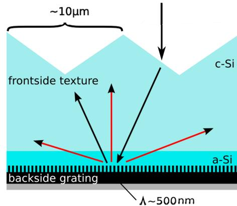
Figure 1: Sketch of a crystalline silicon solar cell with frontside texture and binary backside grating with a period  $\Lambda \approx 500$  nm. The black arrows represent the rays in the case of a simple backside reflector. The red arrows indicate additional light paths that arise from the diffraction into higher orders as a consequence of a backside grating.
