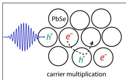
**Figure 1.** A single energetic photon can produce multiple pairs of free charge carriers in a thin film of quantum dots.
