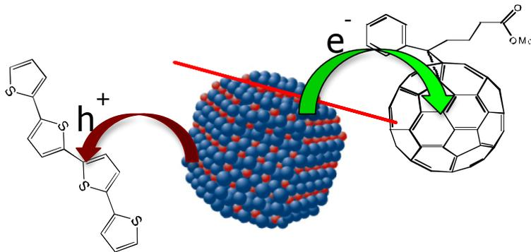
**Figure 2.** We studied the dynamics of excitons in blends of the conjugated polymer P3HT with the electron acceptor PCBM and infrared sensitizing PbS quantum dots.
