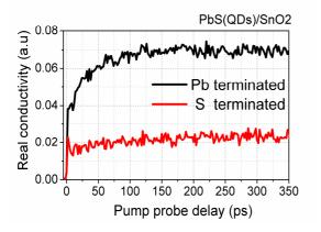
3 fold improvement on the ET efficiency from Pb terminated PbS(QDs) to a SnO2 matrix.
