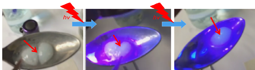
Fig. 2 Light-healing of cellulose hydrogel under irradiation due to photocatalytic reaction and local pH-changes on introduced into hydrogel titania nanoparticles. The light-healing zone is shown with arrows.
