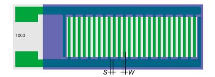
Due to narrow finger width, *w*, and spacing, *s*, (down to 200  $\mu$ m), operation in electrolytes of low ionic strength did not suffer from iR drop, as the underlying conductive patterns of such cells had conductivity cell constants down to 0.008 /cm.
