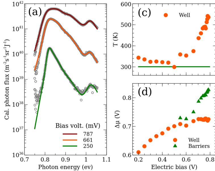
Figures 4 : Variation of carrier thermodynamic properties with bias voltage at fixed laser intensity.
