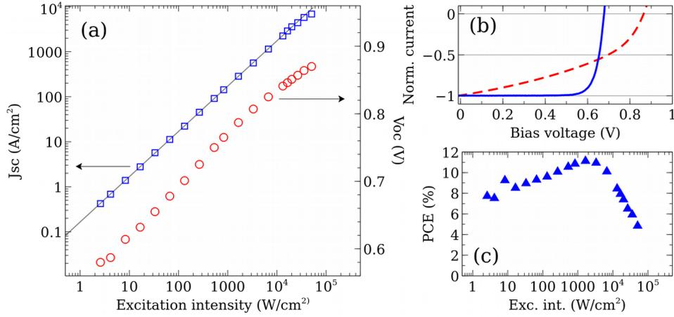
Figure 2 : Electrical properties under different laser illumination. Figure (b) shows two normalized current-voltage curves at low ( $\sim 80 \text{ W/cm}^2$ , blue continuous line) and high ( $\sim 4 \cdot 10^4 \text{ W/cm}^2$ , red dashed line) laser powers.
