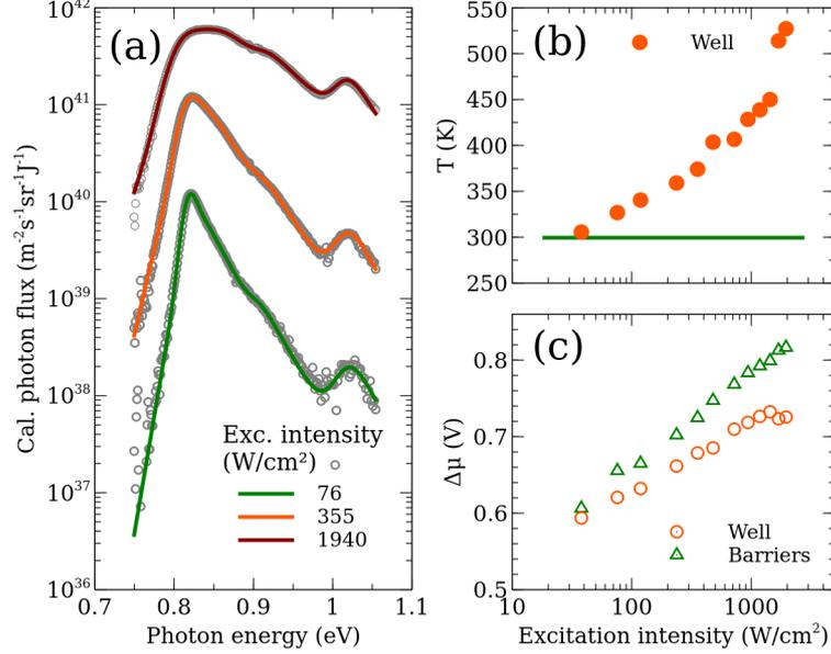
Figure 3 : Variation of carrier thermodynamic properties with laser intensity.
