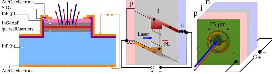
Figure 1 : Device structure and electric contact.
