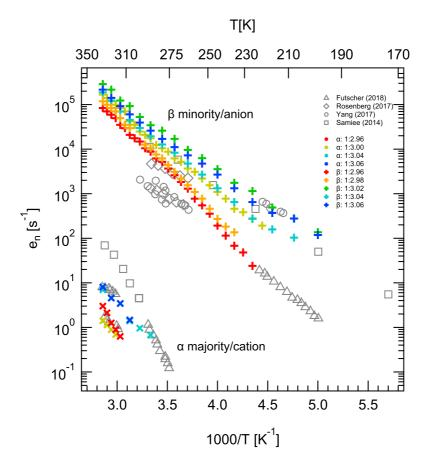
In the stoichiometry varied MA lead halide solar cells, we were able to distinguish two states,  $\beta$  and  $\alpha$ . For comparison, some emission rates from the literature are shown, for different perovskite systems: MA lead halide,<sup>2</sup> single crystalline MAPbBr<sub>3</sub>,<sup>3</sup>  $\alpha$ -phase formamidinium PbI<sub>3</sub> (containing some MAPbBr<sub>3</sub>),<sup>4</sup> and MA PbI<sub>x</sub>CI<sub>1-x</sub>.<sup>5</sup> We expect a lively discussion on our results.
