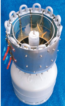
Fig. 1: TPV prototype system. A selective \text{Yb}_2\text{O}_3 emitter, heated by a butane burner, illuminates high efficiency Si solar cells. The upper reflector is removed.
