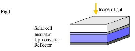
conventional bifacial single junction solar cell. The second main element of the system is the *up-converter*, which partially transforms the sub-band-gap photons transmitted by the solar cell into high-energy photons. The up-converter is electronically isolated from the solar cell and located behind it. A perfect reflector is located at the rear surface of the up-converter.
