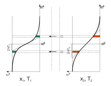
A much larger efficiency is found for thermionic converters. It is due to a barrier for electron emission, the workfunction of the hot emitter, which greatly suppresses transport in the wrong direction at one of the two electrodes of the converter.
