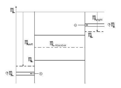
The increasing ability to suppress transport in the wrong direction is the main difference in the conversion of heat into electrical energy by thermoelectric converters, thermionic converters and hot electron solar cells, making the hot electron cell the ultimate thermoelectric device.
