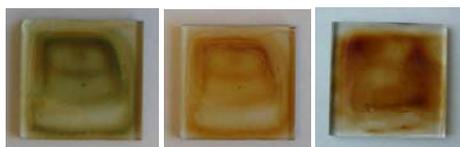
Fig. 1 The appearance of the fresh film from fresh HCl solution (green), HCl films exposed to air for several days (orange) and the basic solution of PTEBSNa (dark orange)
