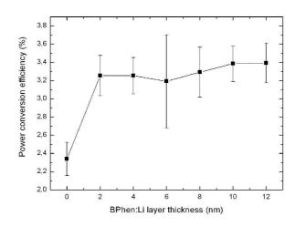
Fig. 1: Lithium doped BPhen layers between the absorption layer and the cathode increase the open circuit voltage, the fill factor and thus the power conversion efficiency of the solar cell. Due to the good electron transport properties, the layer thickness of BPhen:Li is of secondary importance.
