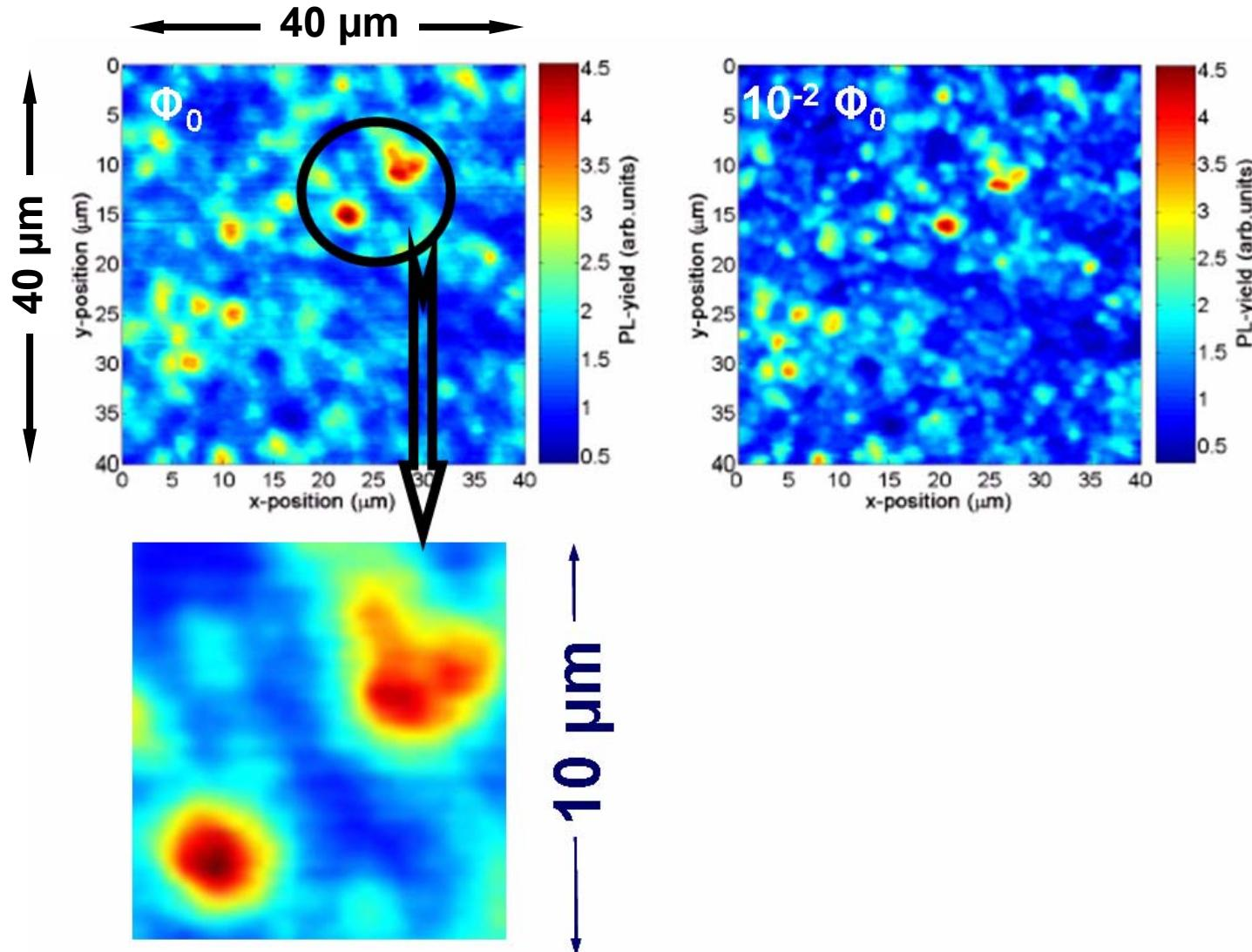
yield of confocally recorded photo-luminescence of  $\text{CuInGaSe}_2$  (L. Gütay et al., 2004)
