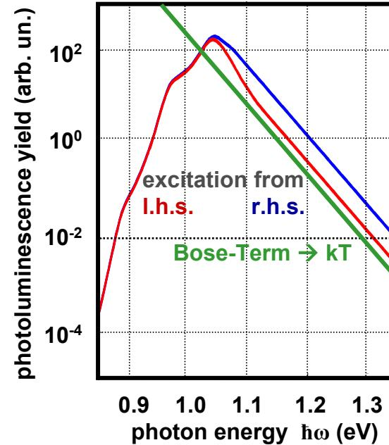
numerical modelling for examination of influence of carrier depth profile on spectral pl
