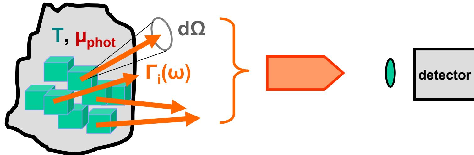
$\Gamma_{\text{tot}}(\omega)$  by integration of over entire volume  $d\Omega$
