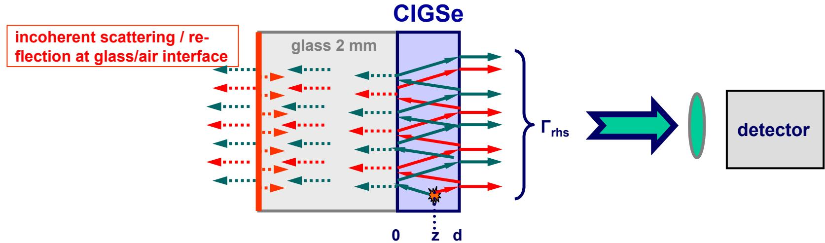
$$\Phi_{rhs}(z) \propto \Phi_B \left\{ (t_{12})^2 \exp(-2\alpha(d-z)) \left| \frac{1 + 2r_{10} \exp(-2\alpha z) \exp[i2kz] + (r_{10})^2 \exp(-4\alpha z)}{1 - 2r_{01}r_{12} \exp(-2\alpha d) \exp[i2kd] + (r_{01}r_{12})^2 \exp(-4\alpha d)} \right|^2 \right.$$
