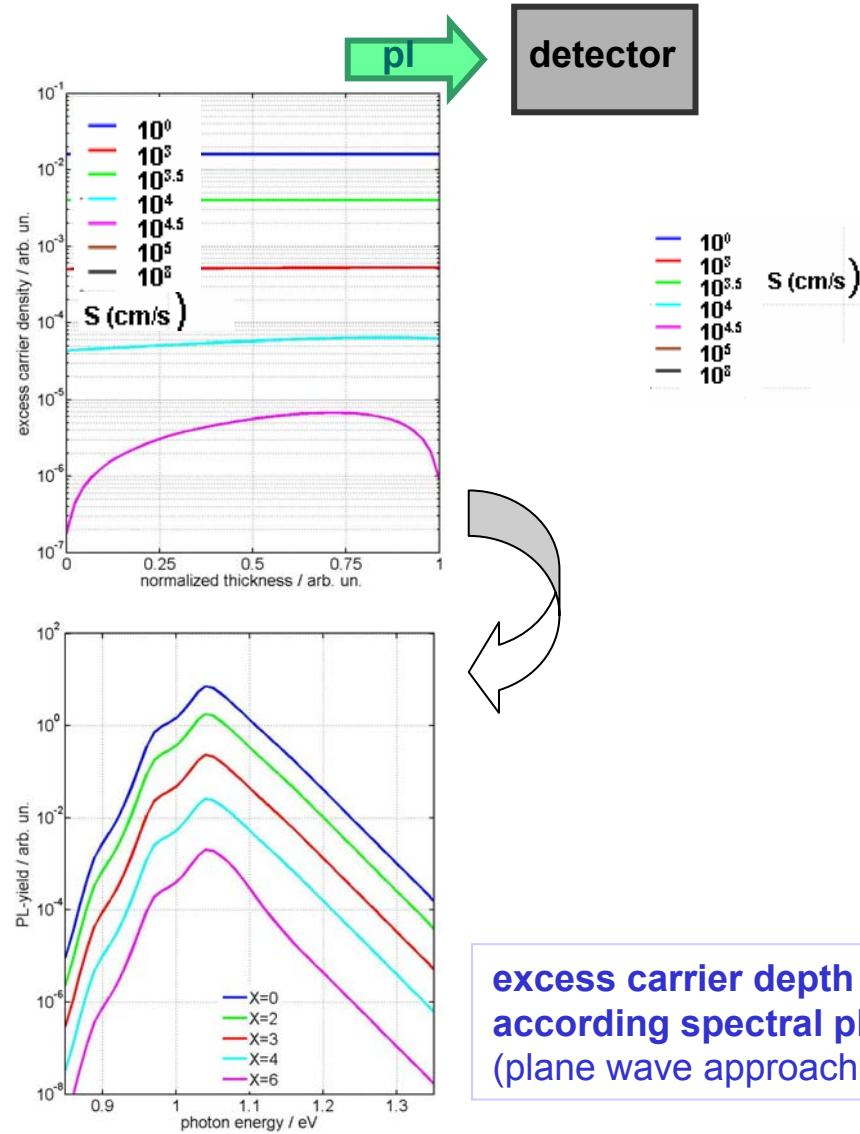
excess carrier depth profiles and
